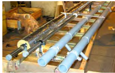
Figure 4. Workshop mock-up of a cabin area pipe module
