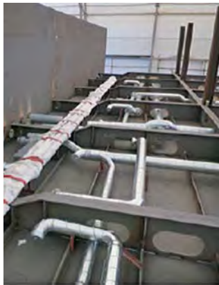
Figure 4. Workshop mock-up of a cabin area pipe module
