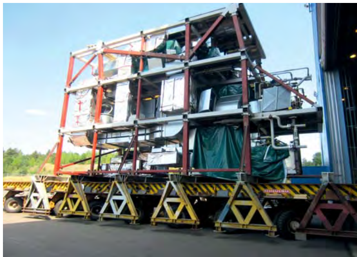
Figure 2. One of the AC room modules ready to be lifted on board newbuilding 1383, Mein Schiff 3
