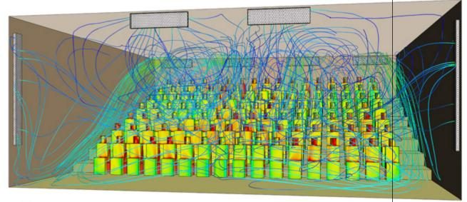
In the picture the audience is colored by contours of static temperature experienced, air motion is visualized by streamlines colored by velocity magnitude.
