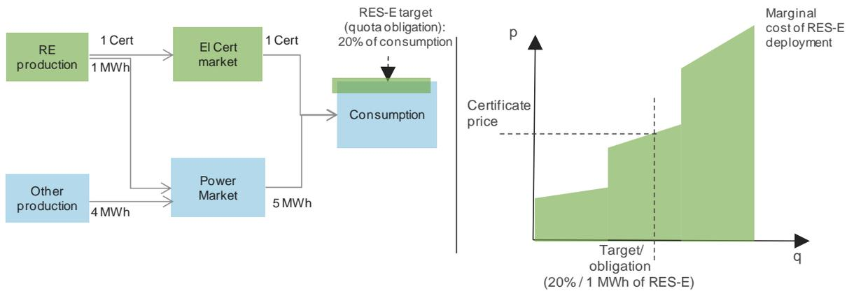
**Figure 1. Basic principle of a TGC scheme (in this illustrative example electricity consumption is 5 MWh and RES-E target 20% of consumption).**
