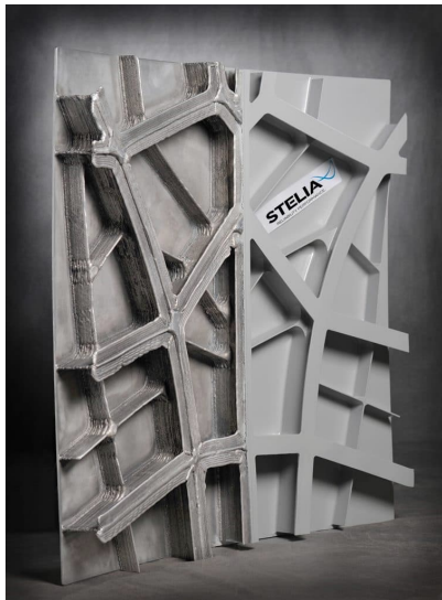
Arc-DED wire: Stiffened Al panel (Stelia Aerospace, France)
