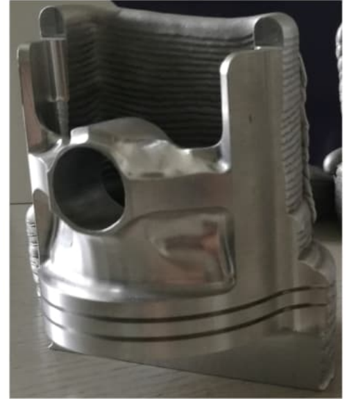
Arc-DED wire: Al 7xxx, motorcycle piston (Klein et al. 2021)
