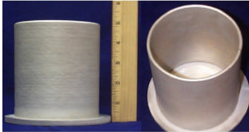
Arc-DED wire (TIG): Aluminum, (Wang et al. 2000, USA)
