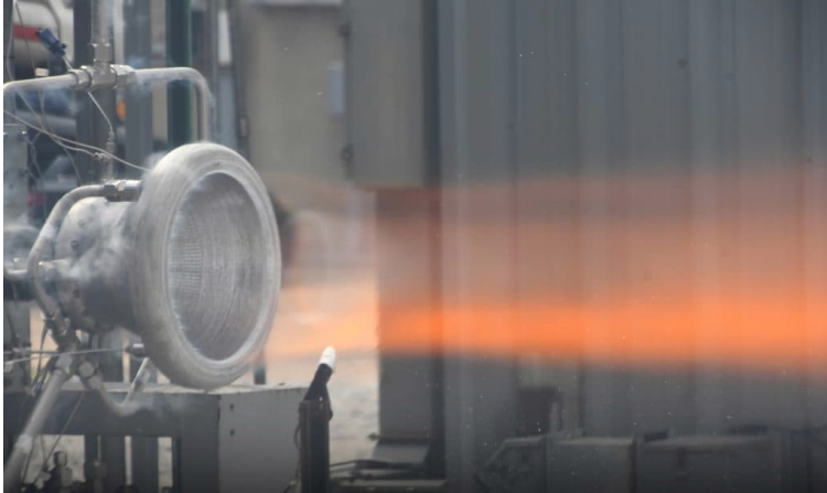
Laser-DED powder: Al 6061-RAM2, Rocket engine nozzle (NASA, USA, 2023)
