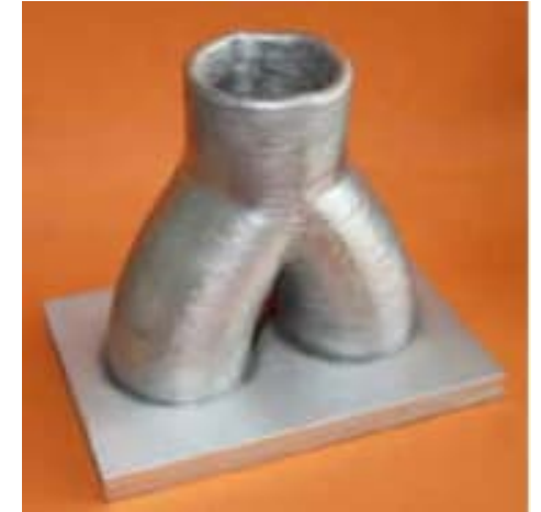
Laser-DED wire: Y branch pipe (Fraunhofer IWS)
