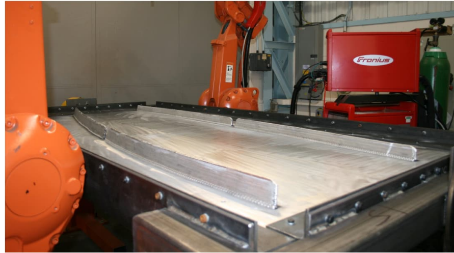
Arc-DED wire: Wing rib, material savings 500kg (Cranfield University, UK)
