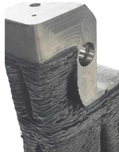
Arc-DED wire: Al 5356, fixing turret (Veiga et al. 2023)
