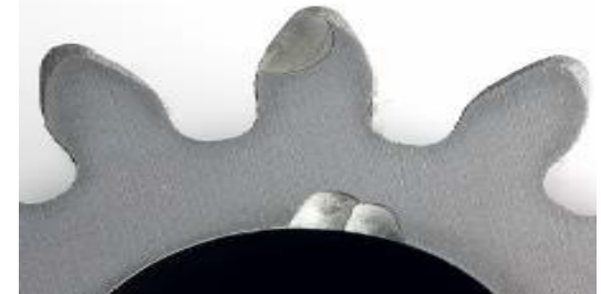
Example: Fineblanking die with chipping
