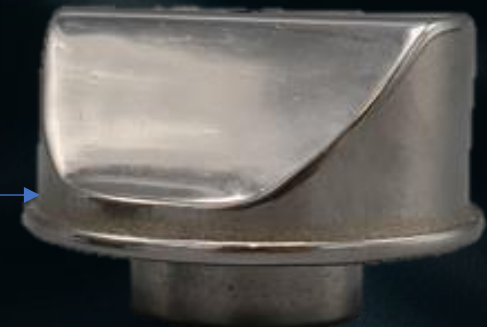
Finished part after tumble polishing
