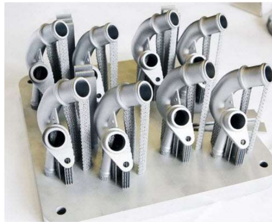
Sample metal 3D printed water connectors for the Audi W12 engine. Photo via Volkswagen AG
