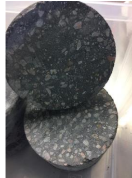
Figure 1. A carbon-negative concrete-like material sample from VTT in 2019 was made using biomass ash, blast furnace slag and green liquor dregs cured with CO 2 . The technology is now commercialised by a VTT spin-off Carbonaide.
